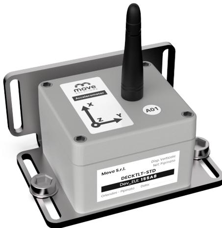
The accelerometer measures the acceleration and temperature of the exact point where it is installed in relation to the structure. It is possible to measure the vibration frequencies and carry out a modal study of the structure. All accelerometers can be perfectly synchronized with each other. Battery power supply and LoRaWAN wireless transmission. The acquisition modes can be set by the user via the web interface provided in the service.
