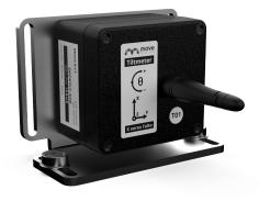
The Tiltmeter measures the inclination and temperature of the point where it is installed relative to the gravitational axis. By installing a system composed of these sensors it is possible to reconstruct the deformation of the structure. All Tiltmeters can be perfectly synchronized with each other, perfect for static load tests. Battery powered and LoRaWAN wireless transmission. The acquisition methods can be set by the user throu-gh the web interface provided in the service.
