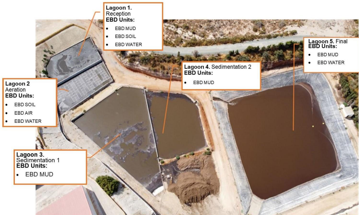
Figure 5.2 Arrangement of the 5 storage lagoons.
