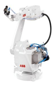
The IRB 52 is a compact painting robot designed specifically for painting small and medium sized parts in a wide range of industries. It provides you with an affordable, professional and high-quality painting solution.
