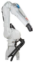
Design for universal backup in moving line and en-hanced solution in stop & go line, IRB 5500-27 offers the increased flexibility and reach to accommodate diverse automotive body sizes, which can potentially reduce the number of robots required on a paint line. This increased flexibility combined with the ability to adjust the robot's installation position reduces cycle times.
