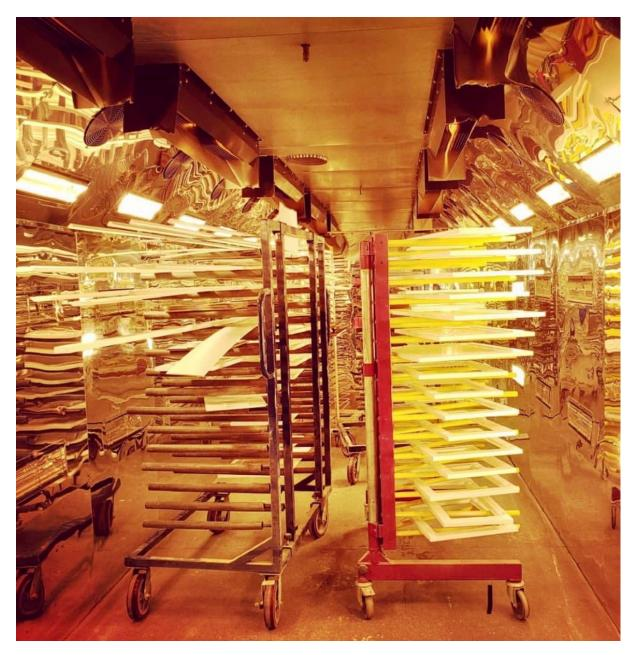
"I didn't see any other way to do it and not kill us in terms of resource issues," he adds. "The halogen lights, the halogen batch tunnel is cool because it has a **laser that detects the temperature of the material**."
