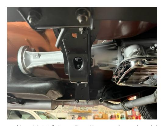
Before the overdrive unit is installed, you will need to measure the coupler end play. Follow their instructions. Our application only required 2 shims to meet the requirement. With the coupler and gasket in place, the overdrive unit is ready to be installed.
