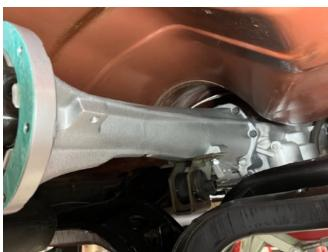
After all the housing bolts are torqued and the snap ring cover plate is installed you are ready to put the transmission mount on the new housing. I used the two new bolts Gear Vendors provided because they are shorter than the factory bolts. Put the frame cross member back into place and torque all fasteners per service manual recommendation.
