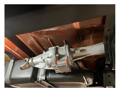
Note: the overdrive unit is fairly close to the gas tank. This will require a right angle adapter, P/N 1S0219 (not included), to allow the speedometer cable to fit without binding. When you place your order for the overdrive inform them that you will need the adapter. Gear Vendors provides an additional length cable with the kit which also connects to a signal generator and then to your original cable.
