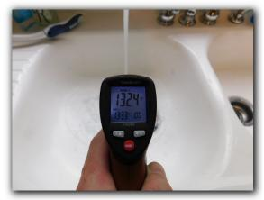
☑ Heated water temperature was observed to be greater than 120 degrees Fahrenheit F and was a SAFETY HAZARD. Adequate and safe heated water temperatures are considered to be between 100 degrees and less than 120 degrees Fahrenheit. The cause of improper heated water temperature should be determined and should be corrected as needed. The water heater thermostats may be turned up too high or there may be other defects in the water heating equipment.
