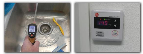
☑ Heated water temperature was observed to be greater than 120 degrees Fahrenheit F and was a SAFETY HAZARD. Adequate and safe heated water temperatures are considered to be between 100 degrees and less than 120 degrees Fahrenheit. The cause of improper heated water temperature should be determined and should be corrected as needed. The water heater thermostats may be turned up too high or there may be other defects in the water heating equipment.
