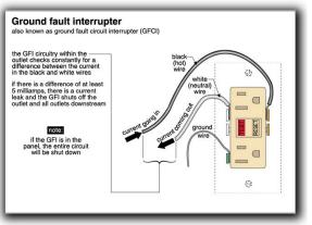
☑ Kitchen counter top electrical receptacles were observed to lack ground fault circuit interrupter (GFCI) device protection. Under current electrical standards, all of the kitchen counter top receptacles should have GFCI protection. Lack of GFCI protection in required locations is a SAFETY HAZARD.
