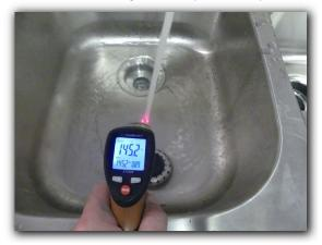
☑ Heated water temperature was observed to be greater than 120 degrees Fahrenheit F and was a SAFETY HAZARD. Adequate and safe heated water temperatures are considered to be between 100 degrees and less than 120 degrees Fahrenheit. The cause of improper heated water temperature should be determined and should be corrected as needed. The water heater thermostats may be turned up too high or there may be other defects in the water heating equipment.
