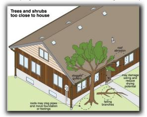
☑ Inadequate clearance between the exterior wall cladding and grade (high soil or mulch) was observed. Inadequate clearance between the exterior wall cladding and grade should be corrected to prevent conducive conditions for wood destroying insects, water intrusion and deterioration of exterior siding materials.
