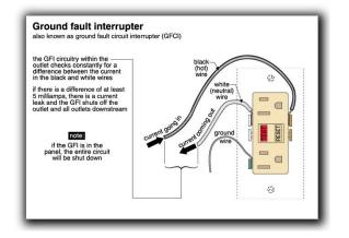
☑ Kitchen counter top electrical receptacles were observed to lack ground fault circuit interrupter (GFCI) device protection. Under current electrical standards, all of the kitchen counter top receptacles should have GFCI protection. Lack of GFCI protection in required locations is a SAFETY HAZARD.
