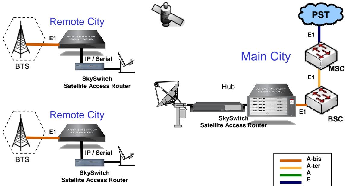
SatPath has brand named this solution “SkyCell” which consist of the seamless integration of SatPath’s SkySwitch Satellite IP Network system and Verso’s Netperformer GSM optimizer. The most important benefit of this solution is the dramatic reduction of Bandwidth expense as compared to other satellite technologies and yet it outperforms them in preserving the functionalities of the GSM Network and the quality of the voice transmission. SkyCell claim to fame statement:
