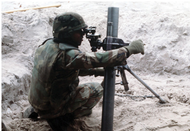
A soldier adjusts the sight line on a M29, 81mm Mortar High-Angle Infantry Heavy Field Mortar. Photo Credit: NARA
