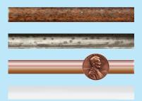
**Lead** - A dull, silver-grey color that is easily scratched with a coin. Use a magnet - strong magnets will *not* cling to lead pipes.
