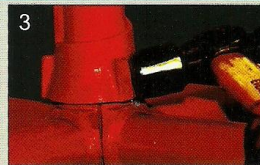
3 Rotate the top cup with hammer to lock the blade ends
