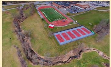
The other project is the Danielle/Willipa Drives Stream Restoration project in Dover Township. This restored 800 LF of an UNT to Little Conewago Creek. Primary purpose of the project was to address resident concerns related to erosion of the stream and loss of rear yards, as well as exposed telephone and cable utility lines. Work involved removing accumulated sediment, filling in washed out areas, constructing rock
