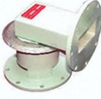
This coaxial part is symmetrically circular, allowing for free rotation without affecting performance. The inner conductor of the coaxial line is usually hollow, allowing further coaxial cables to be put through the wave guide part and to be used with the coaxial modules when building multi-channel rotary joints.
