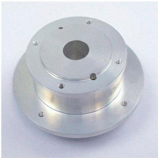
Because coaxial parts are symmetrical in  $\phi$  direction, free rotation without performance degradation is accomplished. In the rotating part, electrical continuity is achieved by  $\lambda/4$ -chokes eliminating metal contacts. The Rotary Joints can have both waveguide ports at a right angle to the rotational axis, 'J-style', one waveguide port at a right angle and one in line, 'L-style' or both waveguide ports in line.
