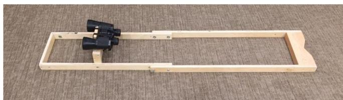
Completed Binocular Support (with bins attached) -
