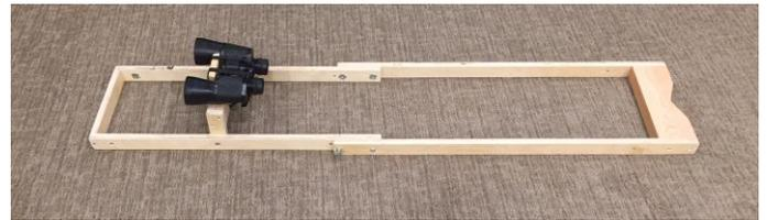
**Completed Binocular Support (with binos attached) -**
