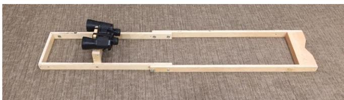
Completed Binocular Support (with binos attached) -
