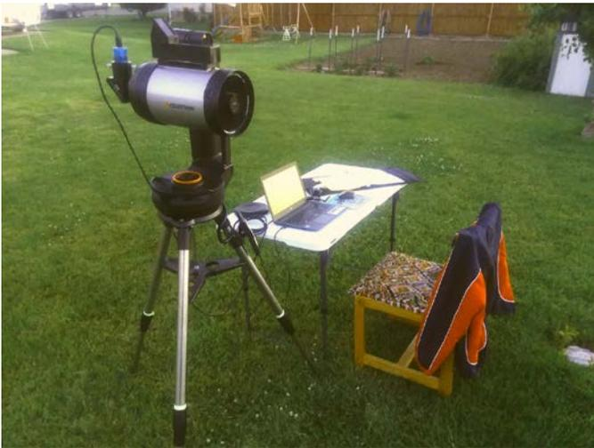
The equipment shown includes a Mallincam SkyRaider DS287/c camera with a 0.5x focal reducer screwed onto the 1 1/4" tube on the end of the camera, and a Meade F/6.3 focal reducer screwed onto the rear cell of my 6 inch Evolution Celestron Scope. This set up gives a nice wide field of view.
