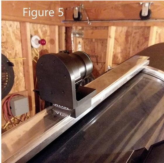
Once I had the Polemaster mounted on my 12 inch tube dovetail I attached a cable that came with it from the camera to my laptop. I had previously downloaded and installed the software from the QHY Polemaster website that controls the camera.
