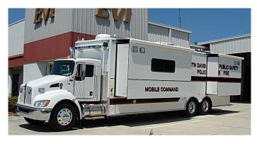
EVI Custom 32 foot Mobile Communications/Command Vehicle Mounted on a Kenworth Chassis. Features two pull out expansion units on drivers side, roll out awning on Passenger side. Multiple radios, desk areas, phones, charging sites, printers, large computer screens, storage cabinets, refrigerator, Generator, Light Tower and many other options built to the departments requirements.
