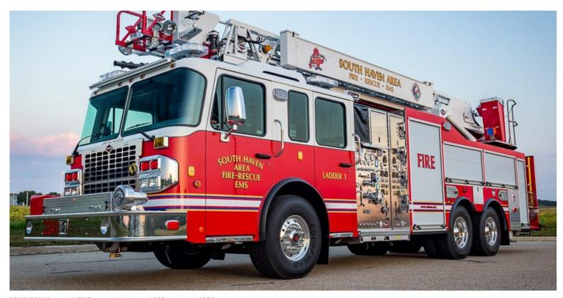
SOLID-POLY Body with 75 Foot straight ladder, 1000 water and 2000 gpm pump
