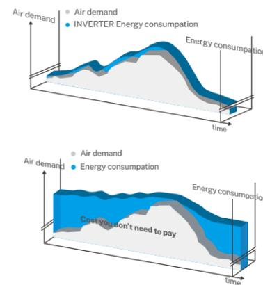
SCR's EPM2 series of compressors adjust compressor's rotating speed depending on the demand, which can change from moment to moment. Thus, it can provide exact volume and pressure what customer needs and achieve maximum energy saving potential. Maximizing energy-saving under any load operation through wide-range inverter control. Wide-range control and Emergency stop function.
