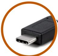
You can't tell what this connector does just by looking at it. It could just provide power, or power + data, or power + video (up to 8K) - or all three simultaneously. Check the specs!
