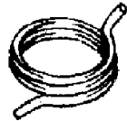
图3-18 云形锁弹簧HB2-54 Fig.3-18 Cloud-like lock spring HB2-54
