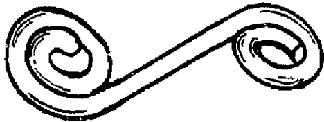
图3-18 云形锁弹簧HB2-54 Fig.3-18 Cloud-like lock spring HB2-54
