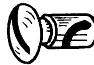
图3-15 扁圆头螺钉HB2-48 Fig.3-15 Oblate round head screw HB2-48
