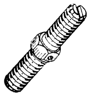
图4-19 拉紧螺栓3HB3-44 Fig.4-19 Holding bolt 3HB3-44
