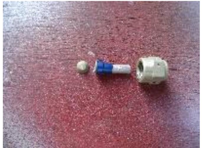
**B-Nut has an un-drilled Restrictor inside**
