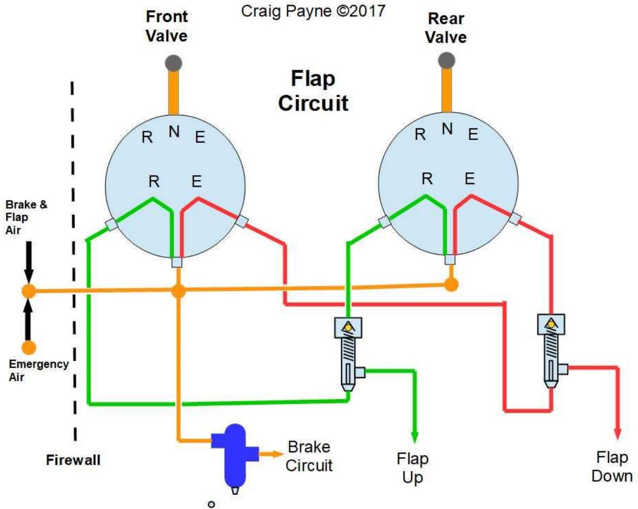
Looking at the Flap circuit, the Rear Valve must be in the Neutral position to allow the Front Valve to function. I safety-wire mine to Neutral but then keep wire cutters in the “ration box” so a **Qualified** back seater could use them in an emergency.
