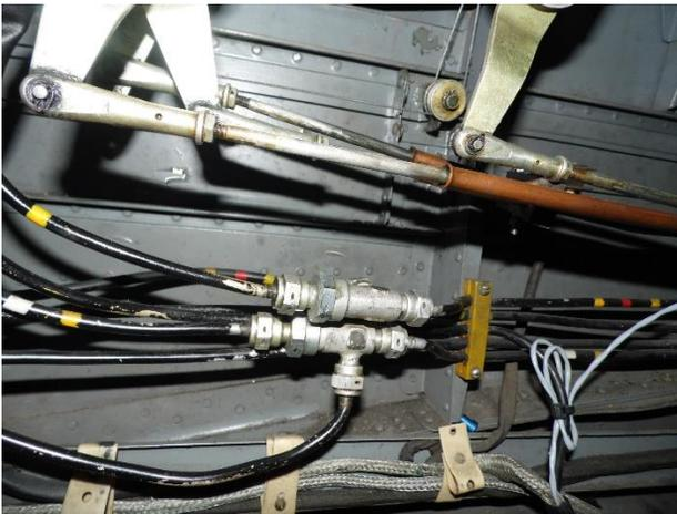
**Flap Diverter Valves in Aft Cockpit**
