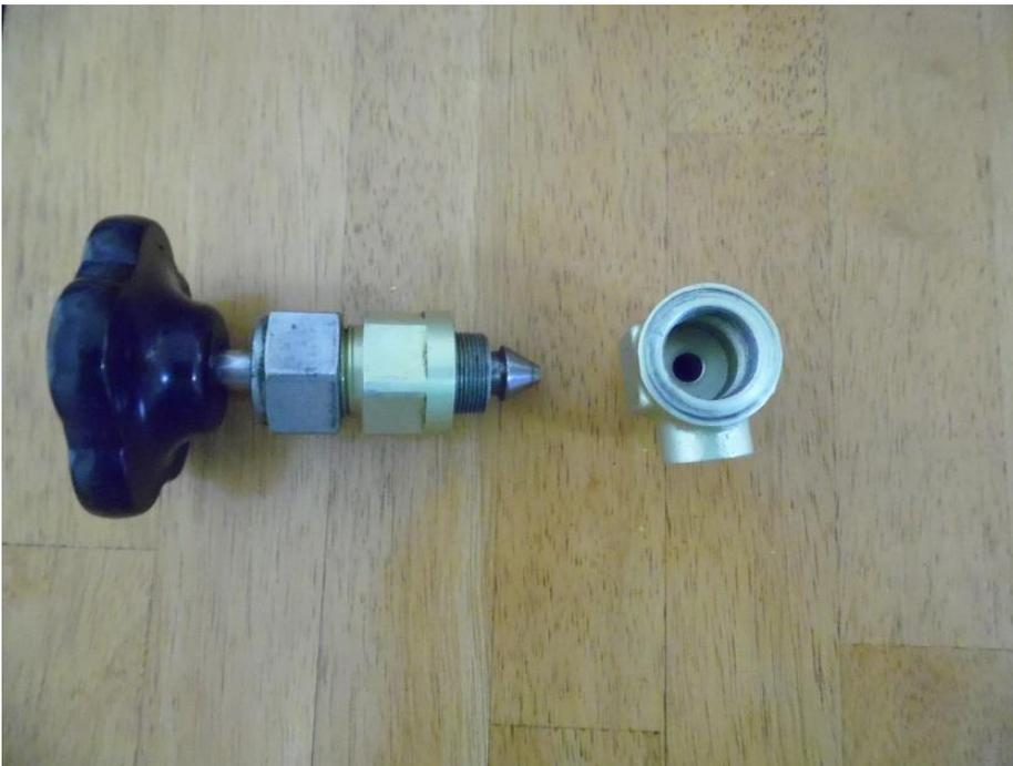
**Air Valve opened** – cone does NOT turn but pushes down into seat. Check for rust & scale if leaking or fails to pass enough air. New, aftermarket Stainless Steel cone shafts are available. Re-plating the cone with chrome also reconditions.
