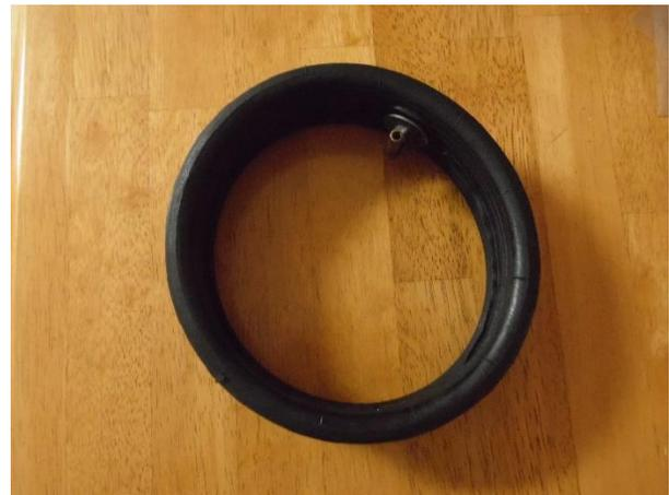
**Brake Bladder** – Heavy rubber pushes against thin metal clips and the brake blocks.
