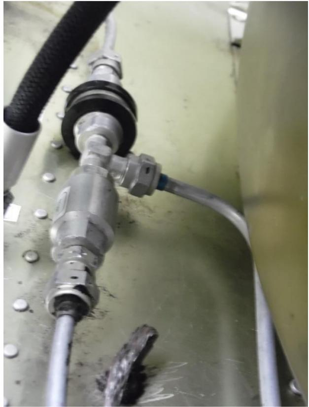
**Right (starboard) Firewall Check Valves (2)**
