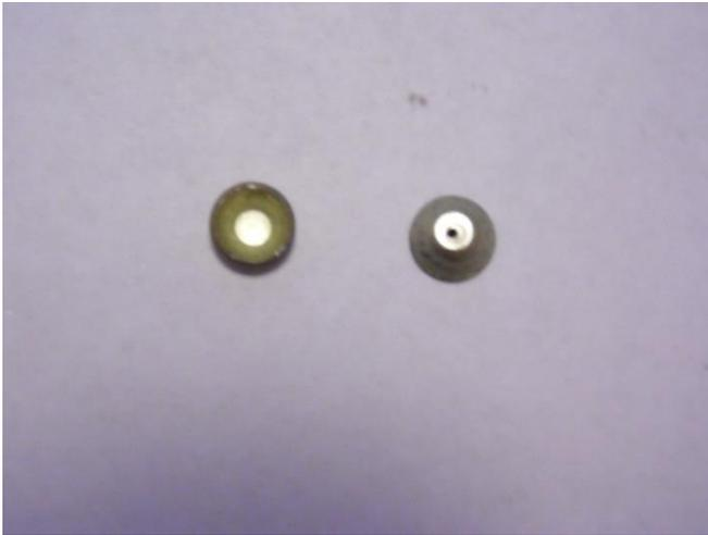
**Drilled and Undrilled Restrictors**
