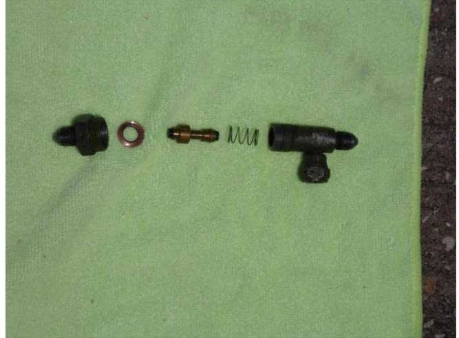
**Gear Diverter Valve** – Steel assembly that can crack due to years of movement with the actuator and hoses.
