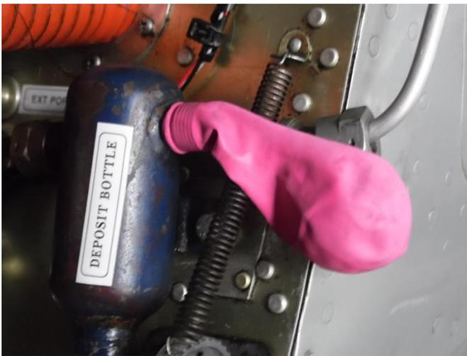
**Balloon Test** – see text for procedure
