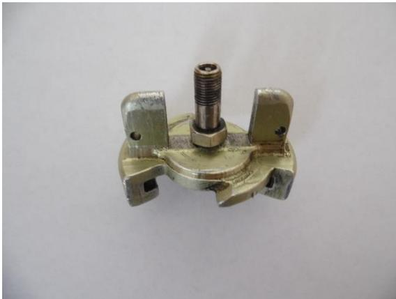
The center of the tab was milled and a 1/8" high-pressure Schrader valve was inserted into the tapped hole. The Schrader will work with or without the actual valve. Without the valve, pressure is contained by the External Fill Check Valve on the firewall. Leaving in the needle valve limits the amount of loss when the fill hose is removed.
