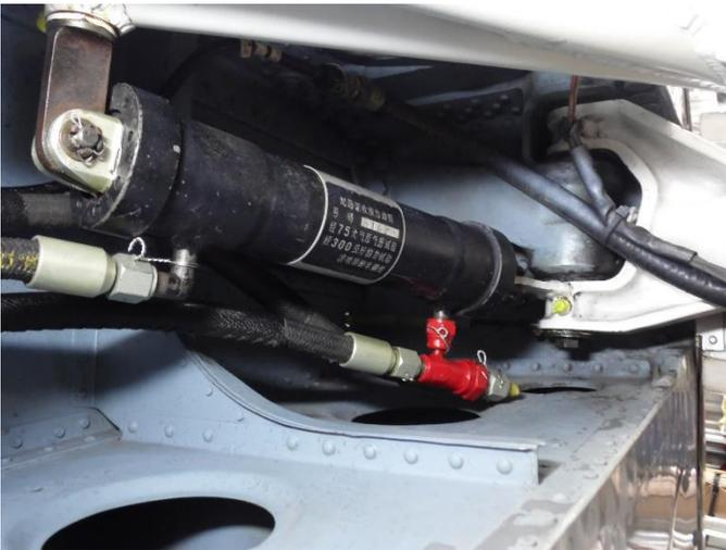
**Main Gear Actuator (diverter valve in Red)**
