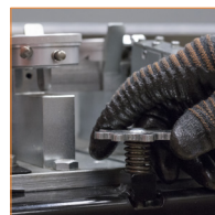
Blade Height Adjustment Knob & Pins Adjust up/down single knob and insert pins for 1"-3" (25 mm - 76 mm) wide blades.
