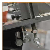
Blade Height Adjustment For 1" - 2" or 1" - 3" wide blades
