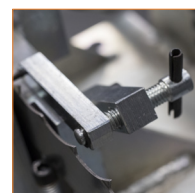
Blade Indexing Pawls Adjusts tooth spacing
