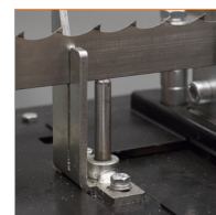
Blade Height Adjustment Knob & Pins Adjust up/down single knob and insert pins for 1"-3" (25 mm - 76 mm) wide blades.
