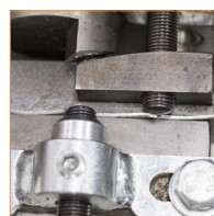
Sets 2 sides at once Efficiently sets both sides in one cycle
