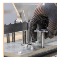
Blade Adjustment Adjust height for 1"-3" (25 mm - 76 mm) wide blades
