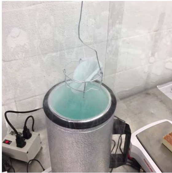
Figure 5. Aerogel specimen under LO 2 boil-off calorimetry testing used to calculate the TCH.
