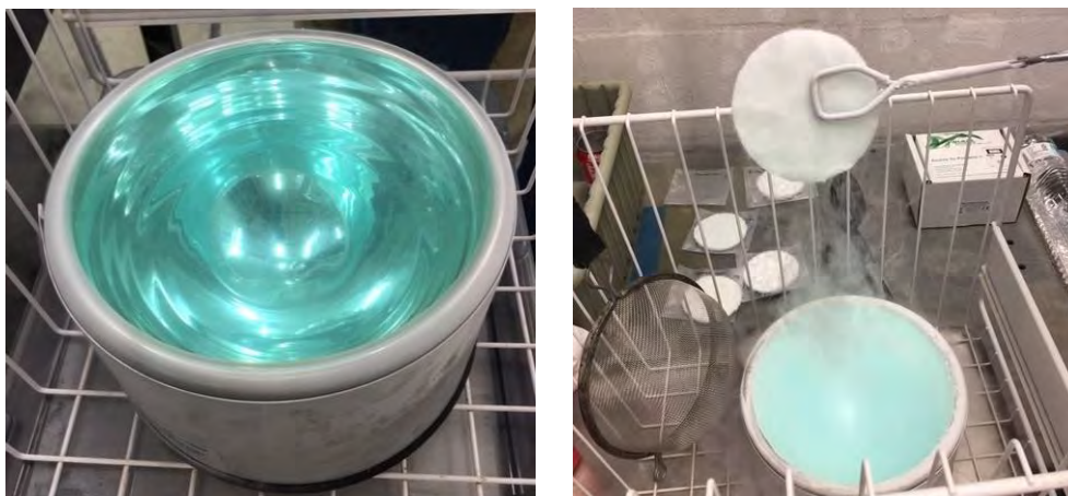
Figure 4. Dewar bowl of liquid oxygen prepared for mass uptake testing of aerogel materials (left); fully charged aerogel specimen being removed from bowl before placement on weight scale (right).
