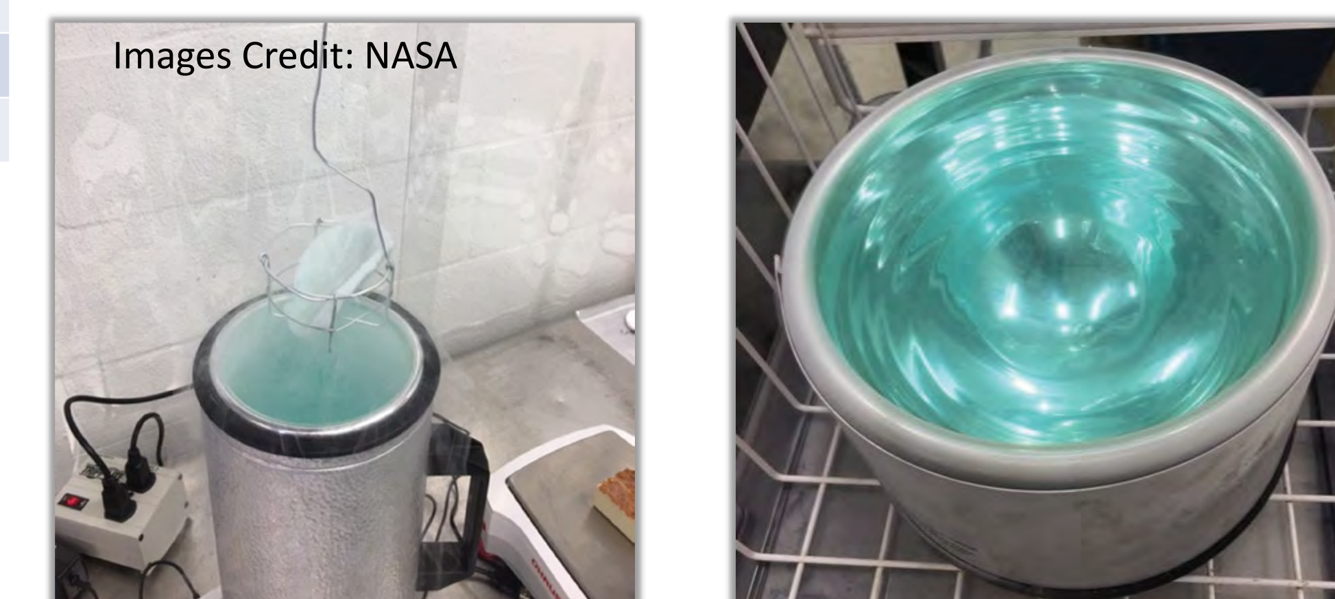
Aerogel specimen under LO 2 boil-off calorimetry testing used to calculate TCH
