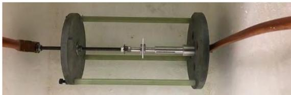
Fig. 4. Electrode and sample configuration for ac electrical breakdown measurement of aerogel insulations at 77 K.
