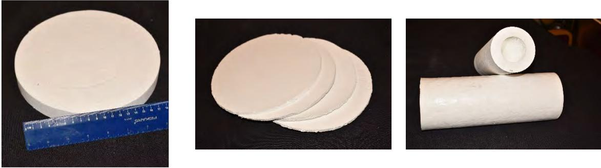
Figure 1. Organic aerogel (a) thick disk stack of thin disks, (b) series of thin disks, and (c) cylinder as cast and after machining into a hollow cylinder.
