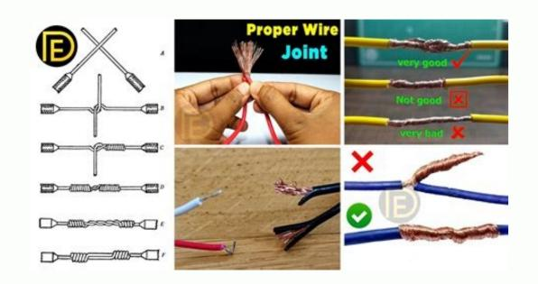
In the following, common electrical cable connections and rat or pigtail connections are listed. This type of connection box. Suitable for processing where no mechanical loads occur and the cables have to be connected to a junction socket, a switch or a Y piece.
