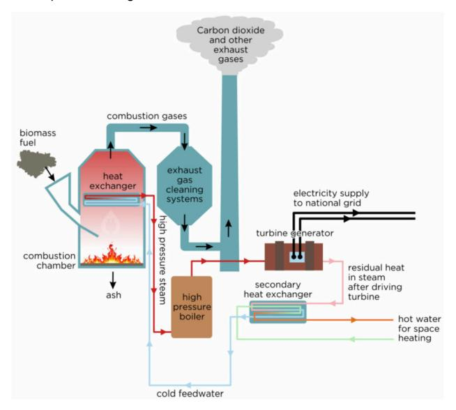
This is called 'Co-generation' or 'Combined Heat and Power' (CHP), and it makes the biomass plant more efficient because the same steam is being used twice to do two different jobs.
