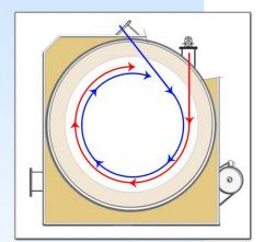
The blue arrows indicate the waste material, and the red arrows represent the initial burner flame to start the process.
