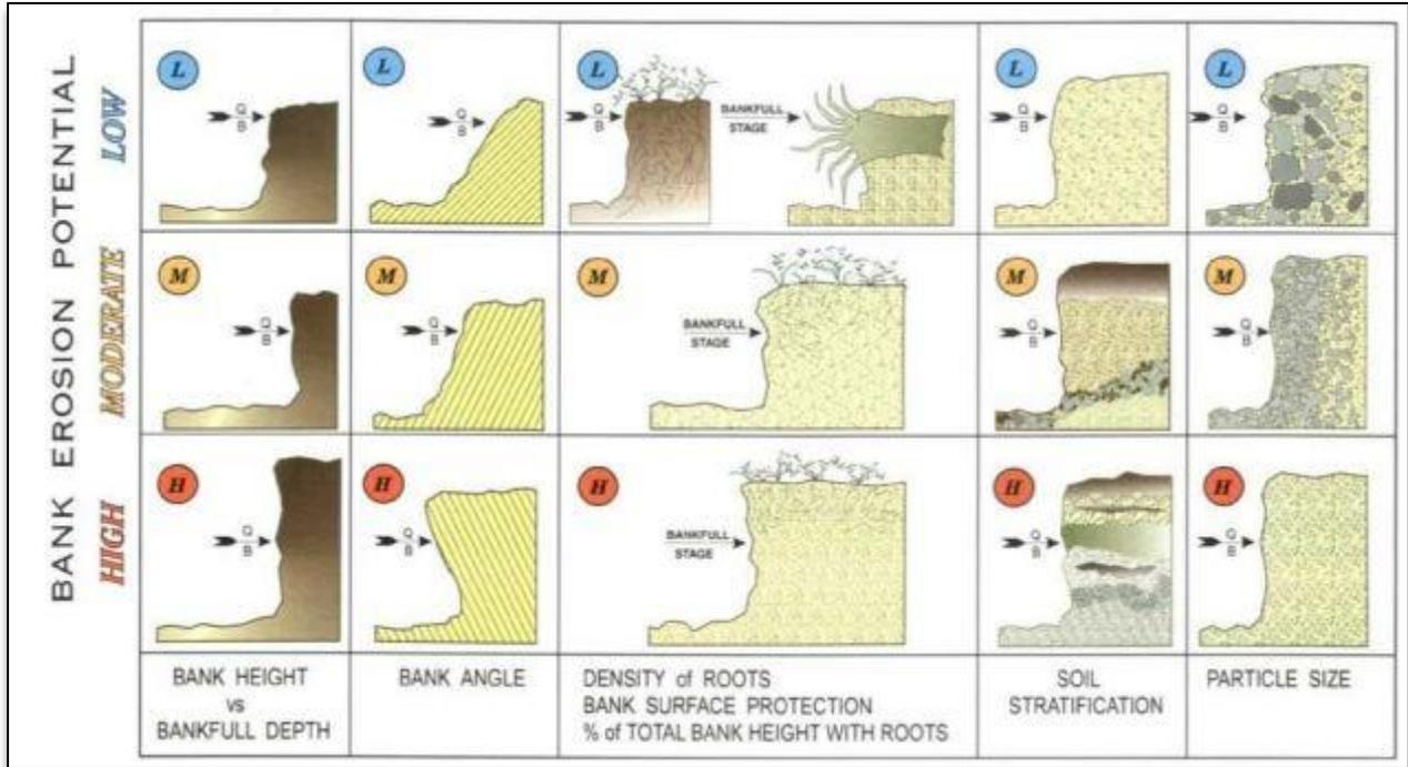
Figure 1. Rosgen Streambank BEHI Erodibility Factors Source: Wildland Hydrology
