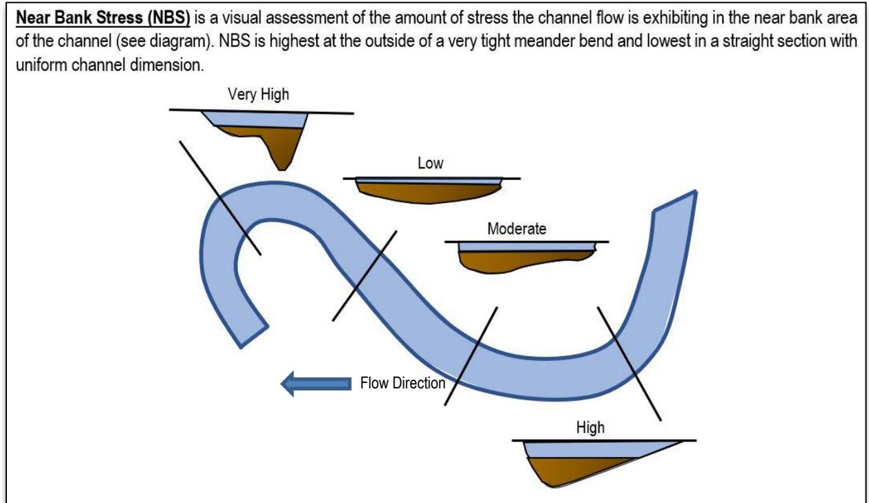
Figure 2. Channel Geometry and Near streambank Stress Classification Source: NCSU RC101
