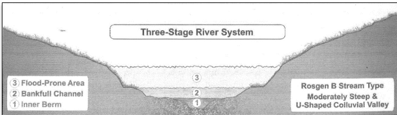
**Figure 3.** Rosgen Priority III three-stage river system Source: Wildland Hydrology
