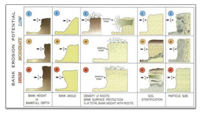
Figure 1. Rosgen Streambank BEHI Erodibility Factors Source: Wildland Hydrology
