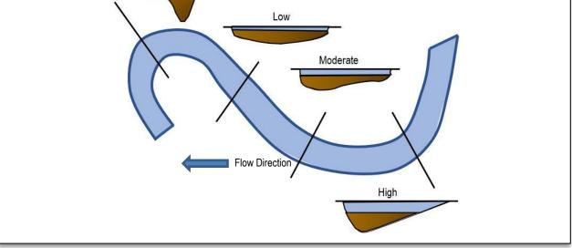
Figure 2. Channel Geometry and Near streambank Stress Classification Source: NCSU RC101
