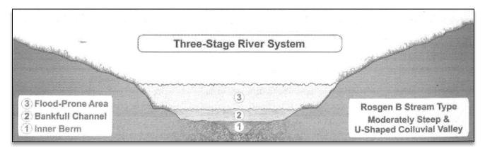
*Figure 3.* Rosgen Priority III three-stage river system Source: Wildland Hydrology
