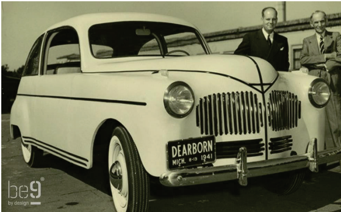
Figure 14 - The Hemp fiber and Soy-plastic car in 1941 being half the weight of steel bodied car from that time.
