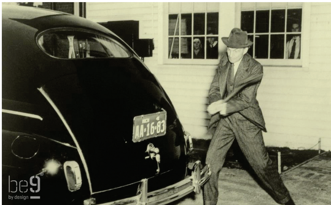
Figure 13 - Henry Ford testing the strength of a Soy-based boot lid with an axe.
