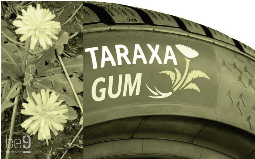
Figure 2: Pioneered in Russia in the 30's, rubber tyres made from Dandelions ( Taraxacum kok-saghyz ). Continental has developed a modern car tyre "Taraxagum".
