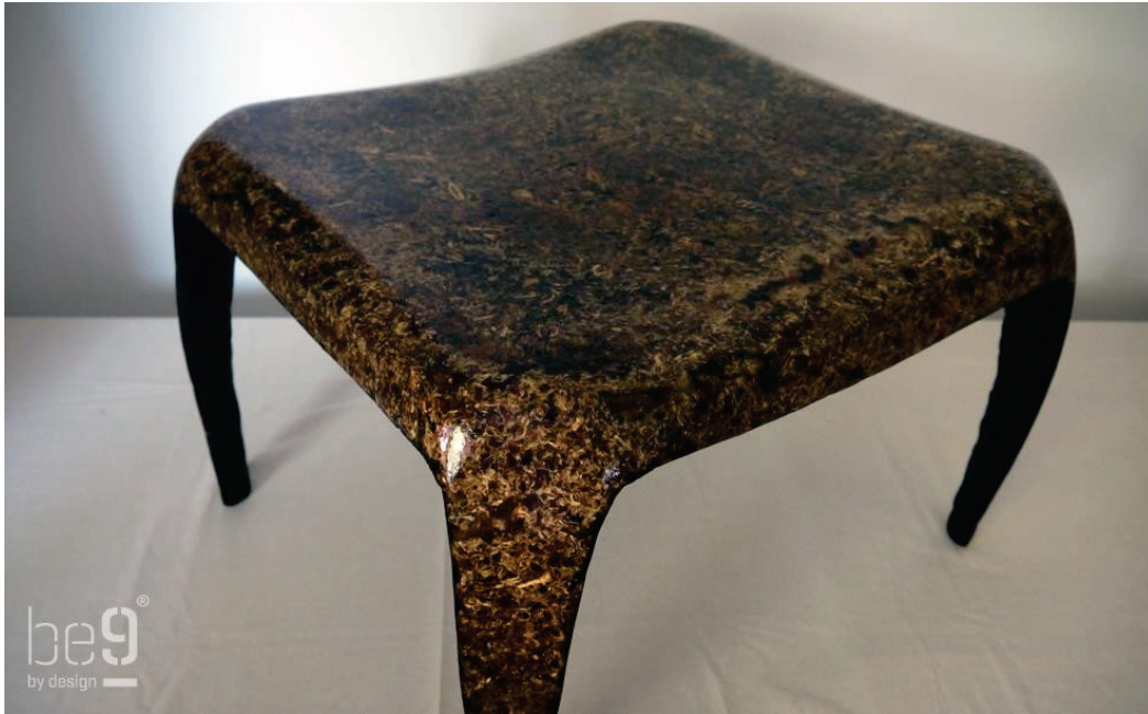
Figure 5: Table made with pinecone chips and a bio-based binder (by author).
