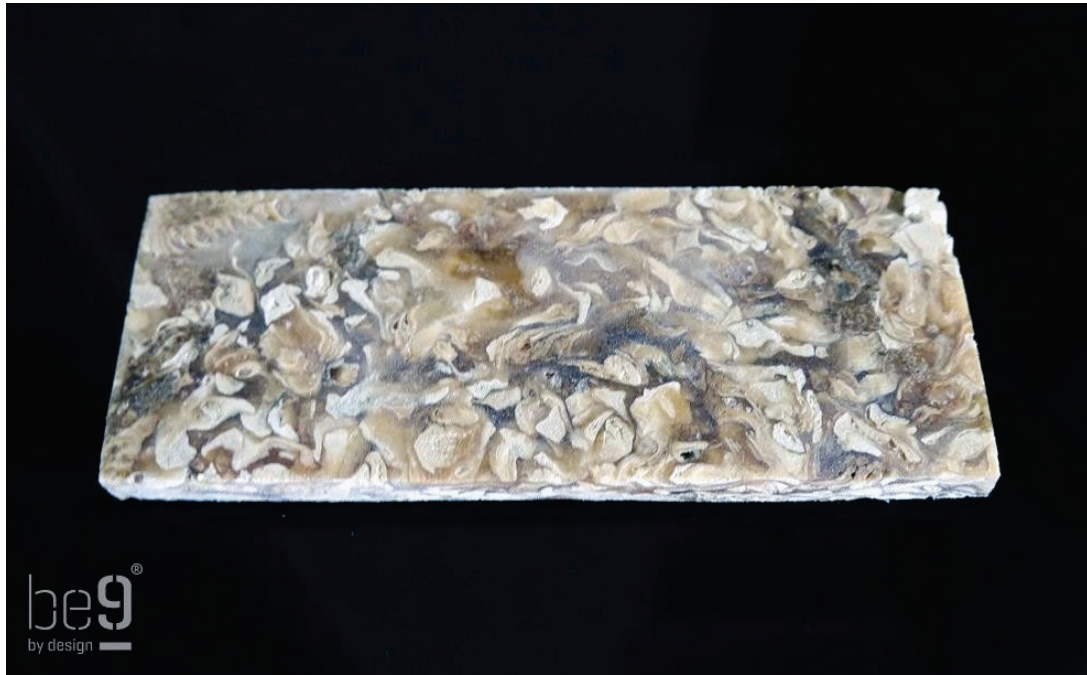
Figure 3: Bleached pinecone chips with a bio-based binder (by author).
