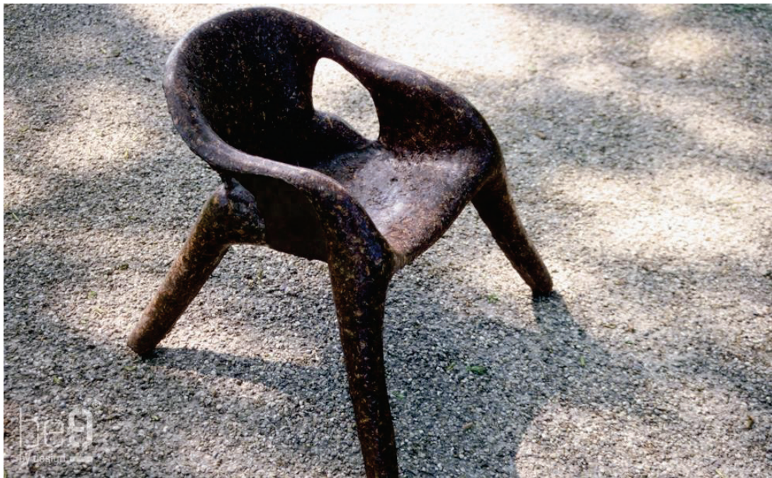
Figure 8: Chair made from pinecone chips and Jute and a bio-based binder (designed by author).
