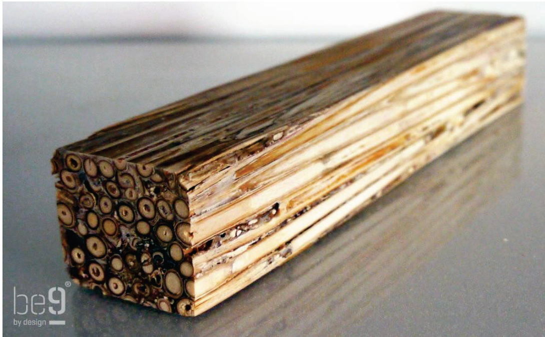
Figure 7: Elephant grass from the garden with a bio-based binder pressed into blocks (by author).
