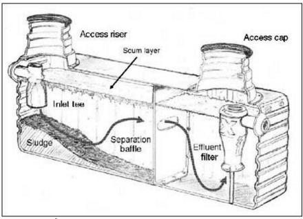
Credit: Éric Brunet, Ontario Rural Wastewater Centre, University of Guelph Figure 2: Common septic tank with access risers and effluent filter
