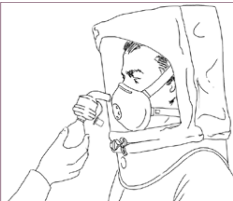
A bitter or sweet solution is sprayed into the test hood for the bitter aerosol or saccharin fit test.
