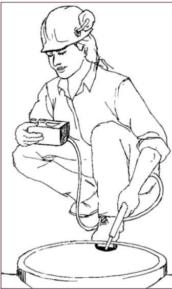
The oxygen level in confined spaces must be tested before workers enter them. Workers must be trained and must follow written confined space entry procedures.
