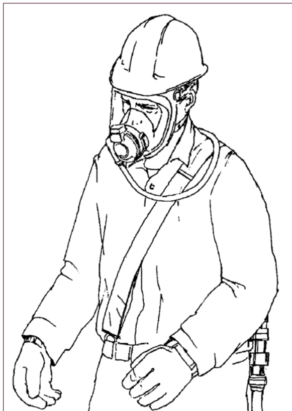
Supplied-air respirators provide clean air through an airline.
