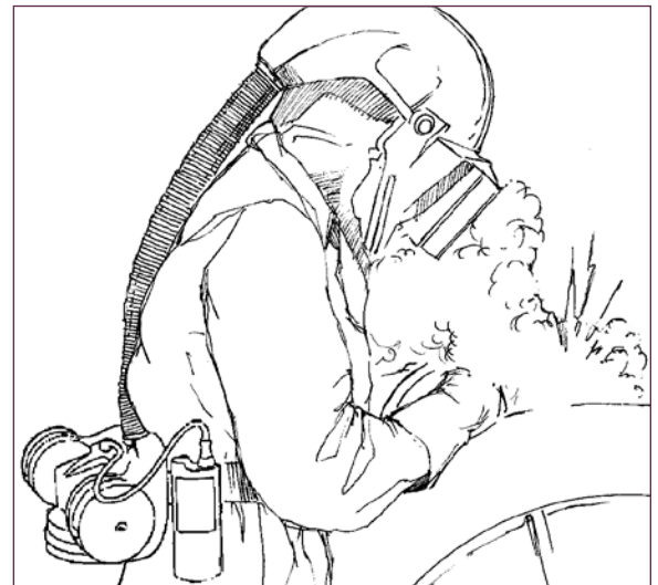
Fumes form when boiled-off material cools and condenses into tiny solid particles.
