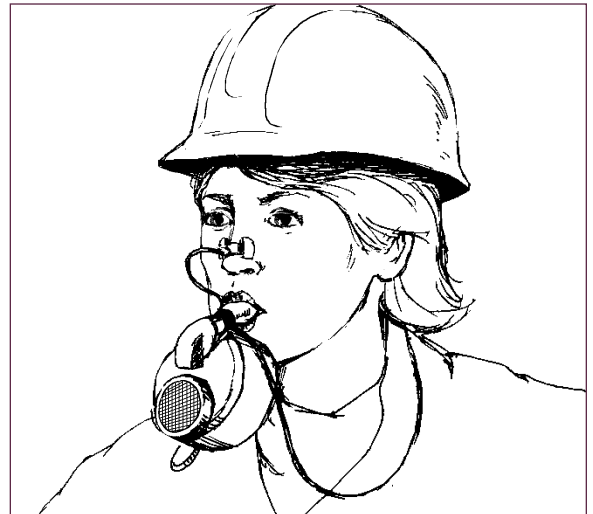
Bite blocks are often used by workers in pulp mills and chemical manufacturing plants.
