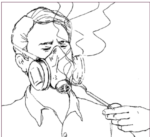
Workers should keep their eyes closed during the irritant smoke test.
