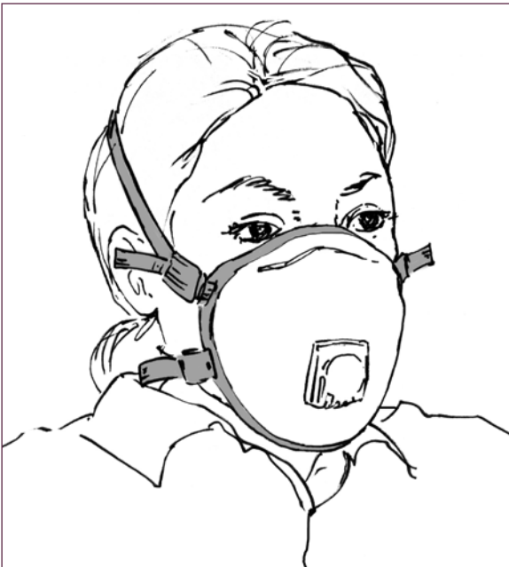
This filtering facepiece respirator has a one-way exhalation valve and an elastomeric edge to give a good seal with the face
