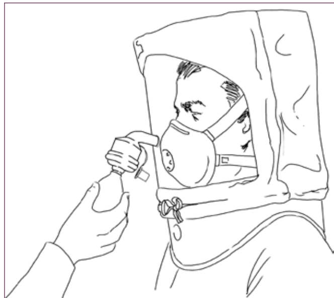
A bitter or sweet solution is sprayed into the test hood for the bitter aerosol or saccharin fit test.
