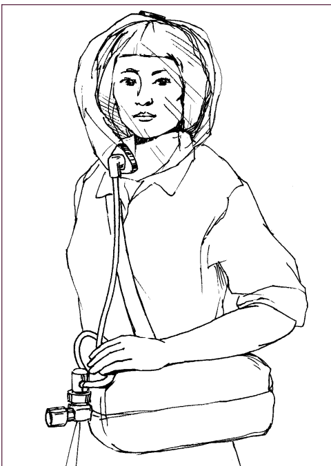
An SCBA-type escape respirator must be used if there is a risk of oxygen deficiency.
