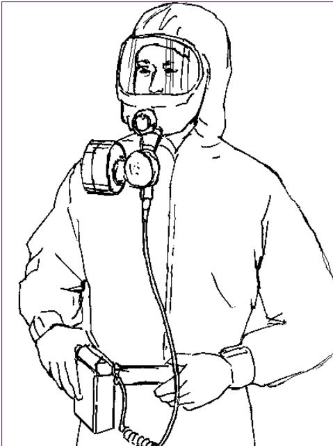
PAPRs use a battery-powered blower to draw air through the filter. This worker is also wearing protective clothing.
