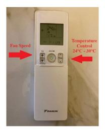
To turn on and off the unit, simply point and press the On/Off button. Then, you can choose fan speed and temperature. Please remember the lowest temperature setting is 24°C in Italy.
