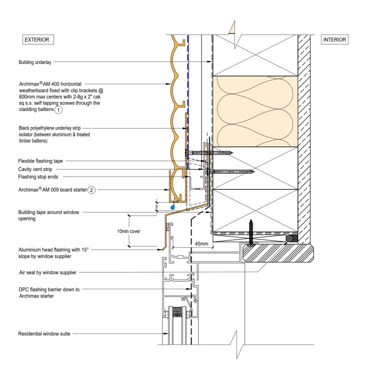
1. Stop ends to be installed at flashing ends
