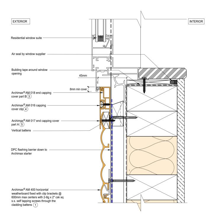
1. Minimum clearance between the AIR BARRIER and WINDOW JOINERY to be 45mm. Window joinery should not be permanently fixed until cladding been installed.
