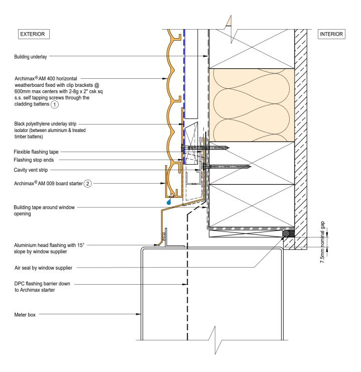
NOTE: STOP ENDS TO BE INSTALLED AT FLASHING ENDS
