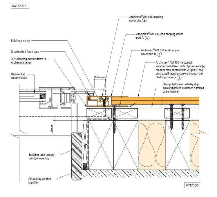
1. Minimum clearance between the AIR BARRIER and WINDOW JOINERY to be 45mm. Window joinery should not be permanently fixed until cladding been installed.
