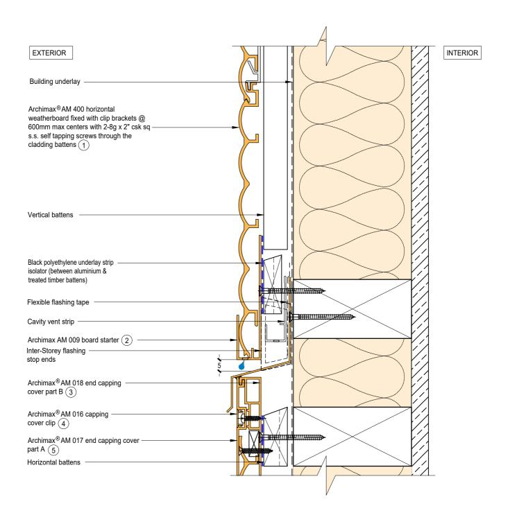
NOTE: STOP ENDS TO BE INSTALLED AT INTER-STOREY FLASHING ENDS
