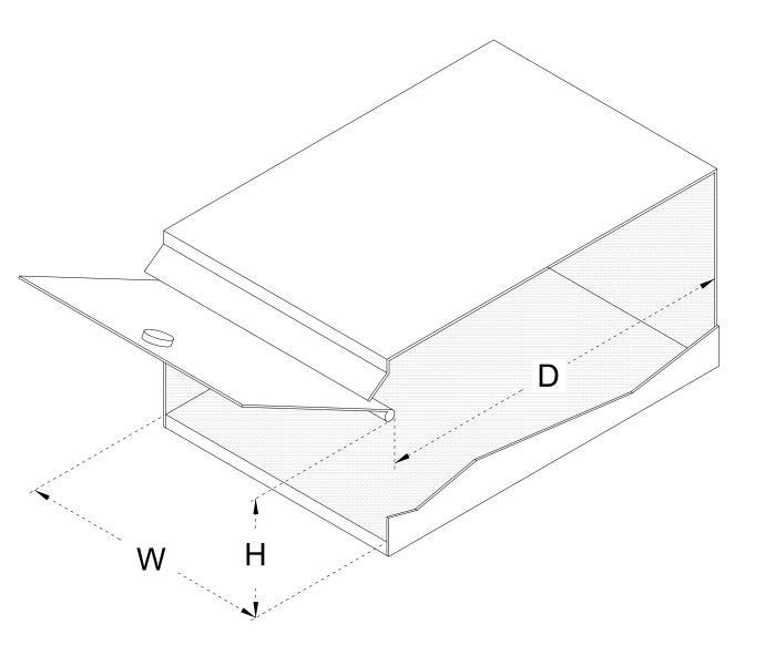
Width = 225mm Min - 250mm Max Height = 95mm Min - 120mm Max Depth = 275mm Min - 335mm Max
