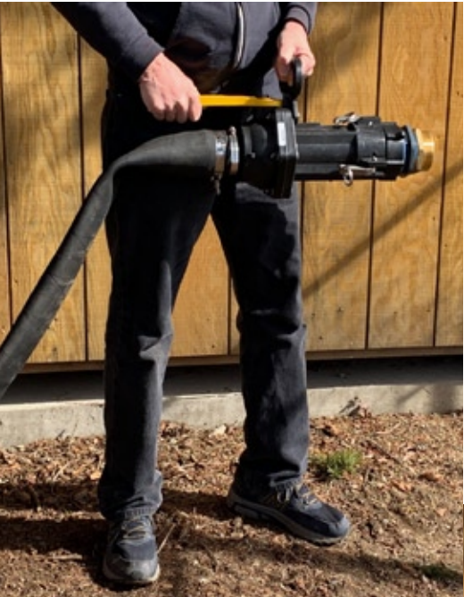
Hand valve with 2.5" m NH fitting
