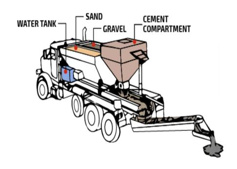
Please Note that the Continuous Auger Mixer needs to be suspended outside the vehicle with a complex hydraulic system for required discharge height.
