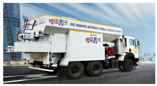
The HAULMIXTM Automatic Mobile Concrete Mixers are provided with a **pollution control Mechanism** automatically operated by PLC during each batch. (Patent Pending).
