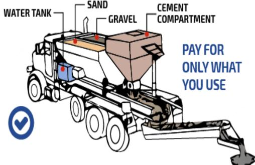
Please Note that the Continuous Auger Mixer needs to be suspended outside the vehicle with a complex hydraulic system for required discharge height.
