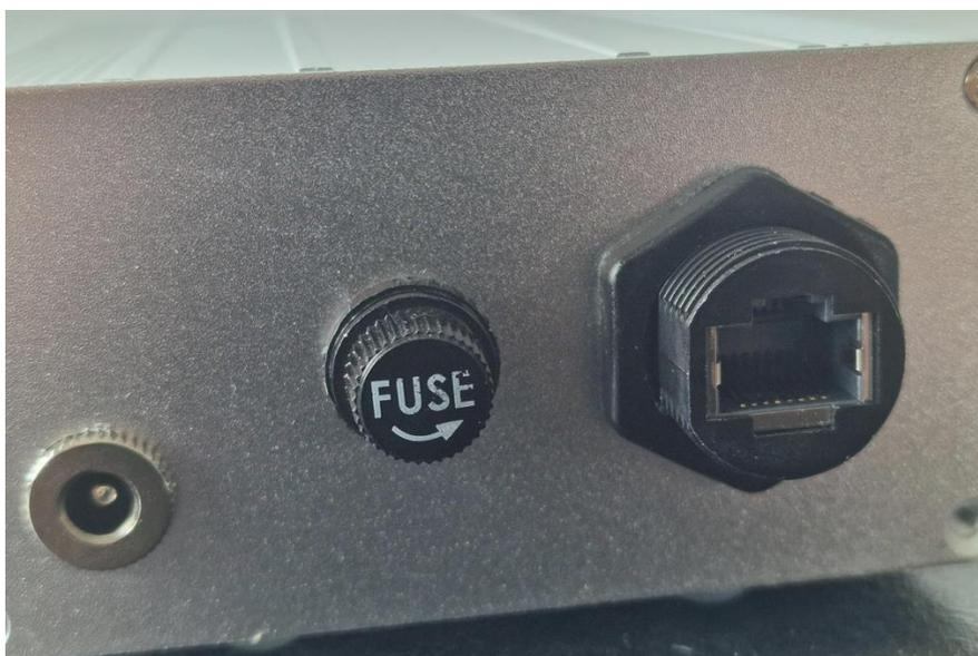
The rear of the switch unit is powered from 12 - 15V DC. The cat cable is connected via the RJ45 socket to the right.
