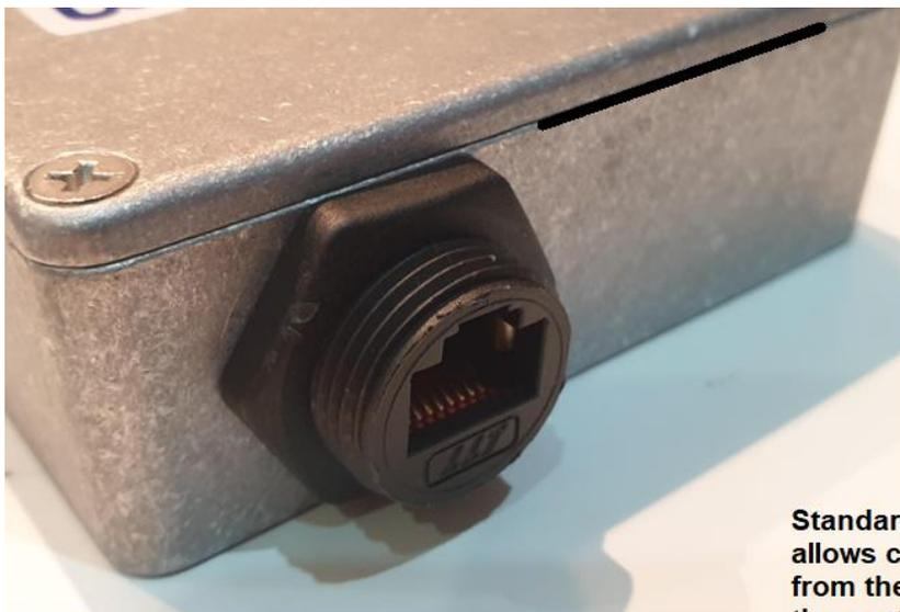
**Standard CAT cable allows control of the relays from the relay box to the control switch box**
