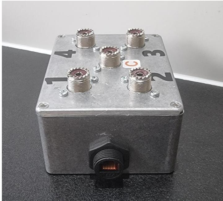
The relay unit is constructed from die cast aluminium and fitted with 5 x SO239 sockets.
